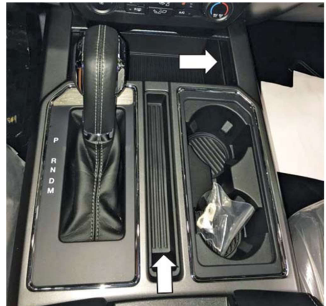
15. Determine a switch location. Remove the panel and drill a 20 mm hole. Route the wires to the switch. (Vehicle equipped with center console shown.) NOTE: Make sure there is enough clearance for the switch behind the mounting surface.
