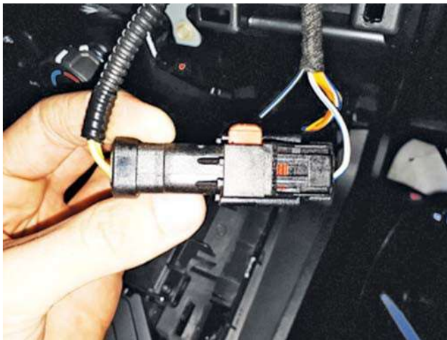
14. Plug the 12V and 110V connectors into the trim panel and leave loose. (The switch can be installed next to the power port if the vehicle does not have the 110V power source.)
