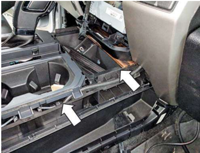
16. Mount the active exhaust on/off switch (FS00056841) in the desired location as shown.
