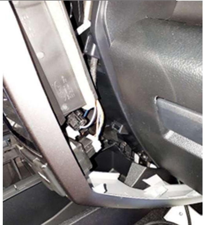
15. Determine a switch location. Remove the panel and drill a 20 mm hole. Route the wires to the switch. (Vehicle equipped with center console shown.) NOTE: Make sure there is enough clearance for the switch behind the mounting surface.
