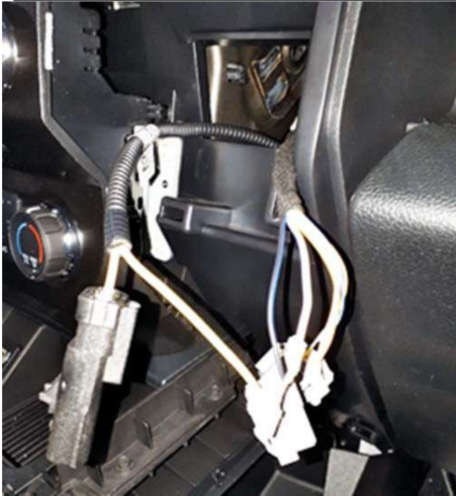
13. Install the supplied connector onto the WHITE with BLUE wire. Connect the mating electrical connectors together. Engage the red locking tab.
