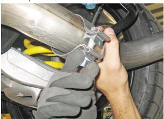
5. Place the band clamp (10-0338) from hardware kit 1315-V8ORRHWK over the exhaust tip and slide the tip over the muffler. Once the tip is in position, torque the band clamp to 30 Nm (Quad Tip shown).
