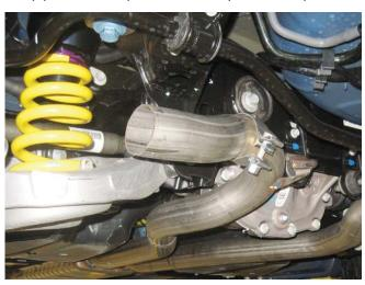
3. Insert the ROUSH muffler hanger into the mount at the rear of the vehicle, and then slide the new pipe over the existing pipe.
