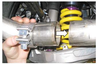
4. Slide the band clamp (94-0053/94-0052) from hardware kit 1315-V8ORRHWK over the joint in step 3 and torque the 15 mm bolt to 30 Nm.
