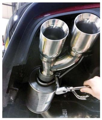
Check the exhaust system for correct clearance under the vehicle and also for tip alignment as shown below. If alignment is off, loosen the required band clamp, adjust, and re-torque the band clamp. (Quad Tip shown).
