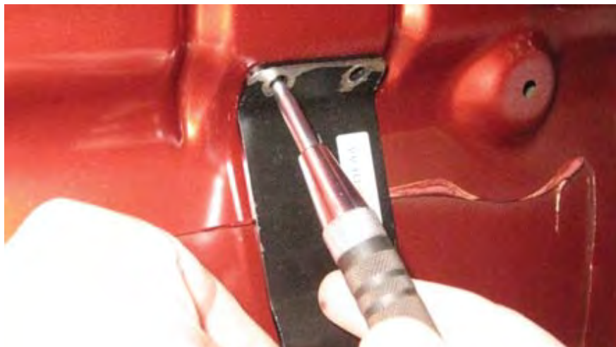
Step 3 Continued - Center Punch Process
