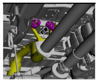
7. Reinstall the factory fasteners using 15 mm socket. Torque to 55NM after the whole assembly is installed.
