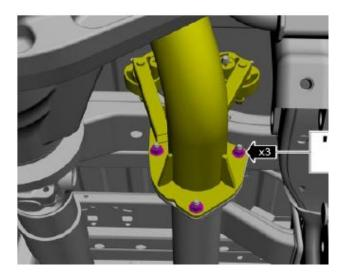
3. Remove 4x rear muffler tailpipe isolator bolts using 10 mm socket.
