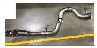
6. Install over axle pipe (1818-5G265) locating to the two hangers.
