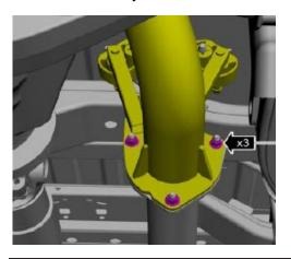
8. Install the tailpipe-tip assembly (1818-5E292DPF) onto the over axle pipe using clamp 2-8-AA and locating off the hanger. Make sure the pipes are installed to the most possible depth and covering the notch. Make sure clamp is roughly 90 degrees to notch (shown above). Torque to 55NM after complete assembly installed.
