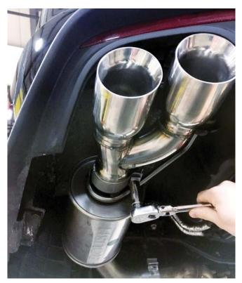
Check the exhaust system for correct clearance under the vehicle and also for tip alignment as shown below. If alignment is off, loosen the required band clamp, adjust, and re-torque the band clamp.
