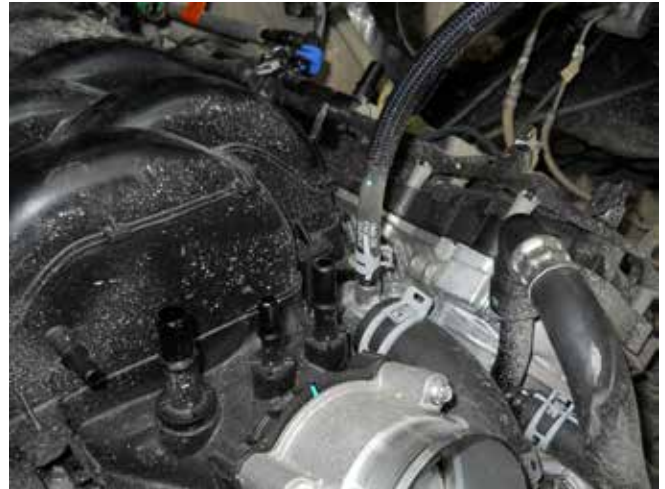
17. Disconnect degas upper bottle-to-radiator hose.
