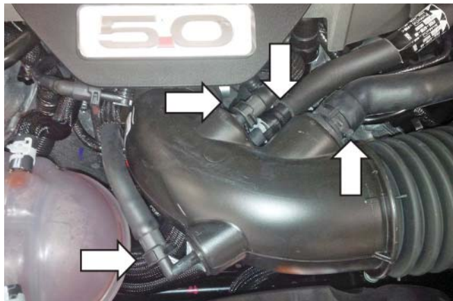
13. Using a 10 mm wrench or deep-well socket, remove the nut retaining the induction resonance tube to the firewall behind the driver side cylinder head.
