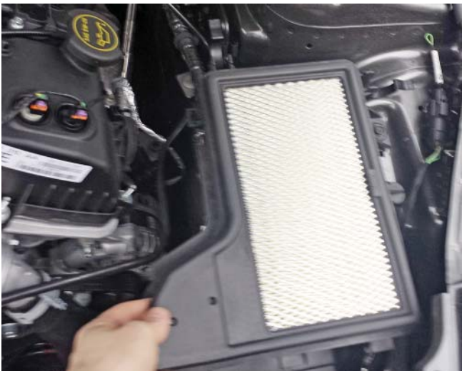
9. Using the 10 mm socket, remove the bolt holding the air box to the inner fender. Retain the bolt as it will be used during installation.
