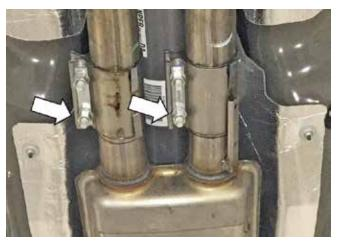
Push the rear exhaust pipes out of the way as needed and remove the resonator. This concludes the removal process for the OEM resonator.
