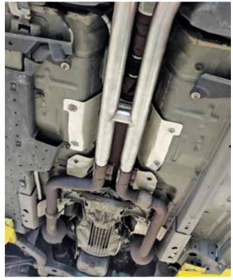
Before starting the vehicle, make sure to check all wires, hoses, brake lines, body parts, tires, and any other components for safe clearance from the exhaust system.
