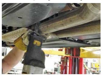
Loosen both of the OEM sleeve clamps in front of the resonator. These clamps are to remain on the vehicle.
