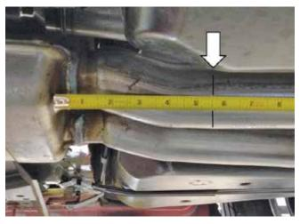
Cut the LH and RH exhaust pipes at the locations marked in step 1 using a suitable cutting tool.
