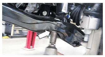
12. Remove and discard the three (3) upper shock absorber and spring assembly nuts from each shock tower. Remove each shock absorber and spring assembly.
