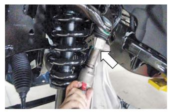
9. Remove and discard the nuts from each lower ball joint using a \_mm socket and remove each spindle. If necessary, use the Ford separator tool.
