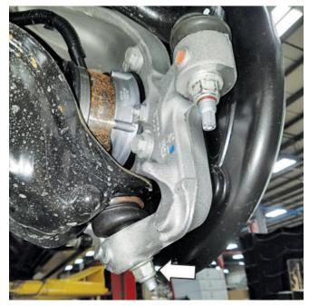
10. Remove and discard the upper nuts from each front stabilizer bar link.
