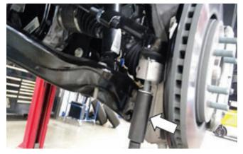
7. Remove the three (3) fasteners retaining the integrated wheel end (IWE) actuator at the end of each front axle.
