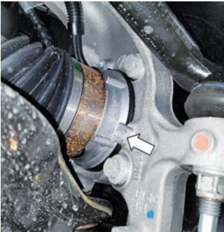
8. Remove and discard the nut from each upper ball joint. If necessary, use the Ford separator tool to remove the ball joint from the spindle.
