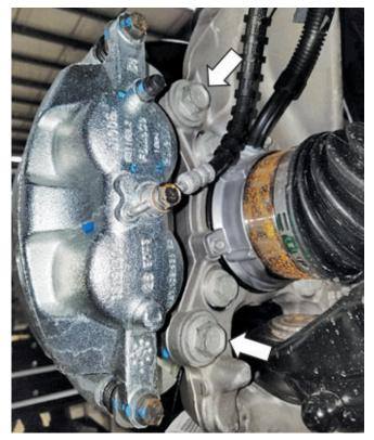
4. Remove the fasteners that retain the front wheel speed sensor brackets and then unclip the front wheel sensor wires from the retainers.
