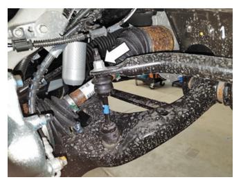
11. Remove and discard the two (2) lower shock absorber and spring assembly nuts from each lower control arm.
