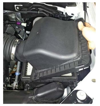
8. Remove the clean air tube from the vehicle.
