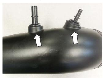
Install couplers and clamps onto the clean air tube (P/N: 111550-9B660) as shown. Tighten the clamps retaining the coupler to the tube to 3 Nm. Leave outside two (2) clamps loose (couplers: right P/N: 111550-9B662, left P/N: 111550-9B662) (clamps: right P/N: R07130015-13, left P/N: 308707426).
