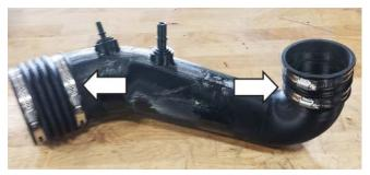
9. Install the clean air tube assembly between the throttle body and the air box. Tighten the clamps to 3 Nm.
