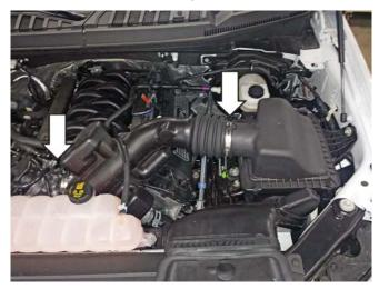
5. Disconnect the two (2) quick connect fittings from the clean air tube.
