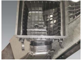
13. If necessary, remove the two (2) rubber grommets from the bottom of the air box and reinstall them into the tray below the air box.
