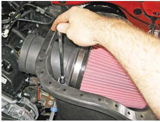
Install the rubber grommet (P/N: 1150-58GRMT) and fittings into the clean air tube. You will want to use soapy water or glass cleaner to aid the installation (fittings: left P/N: 1311-9N285, right P/N: KLR-9N285).
