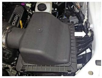
4. Loosen the hose clamps retaining the clean air tube to the throttle body and air box lid.
