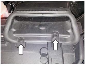
10. Remove the lower air box and dirty air duct from the vehicle.
