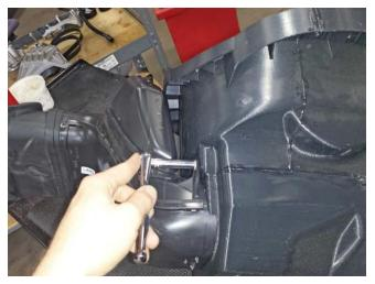
2. Reinstall the bolt, grommet and sleeve into the driver side fender. Tighten the bolt to 17.5 Nm.
