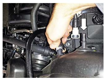
6. Release the two (2) clamps on the front of the air box.
