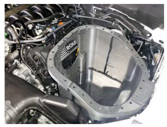
4. Install the air filter (P/N: 131550-9601R) onto the filter tube (P/N: 111550-12B579) and tighten the clamp to 3 Nm. Make sure the filter is installed (as shown) with the metal rib down.
