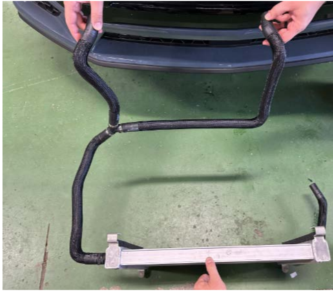
Top View Orientation - LTR Sub-Assembly
