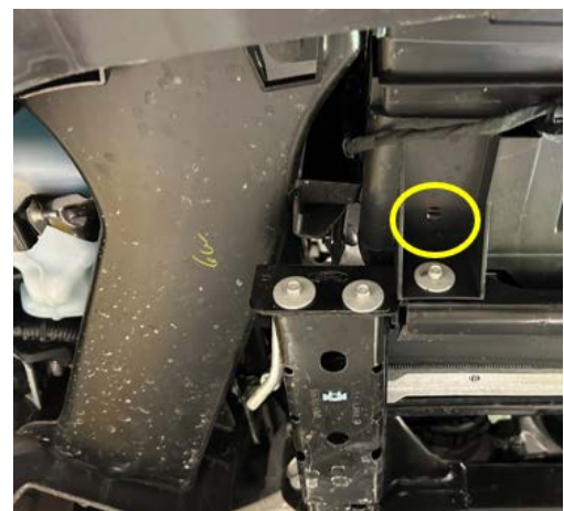
Passenger Side cut hole
