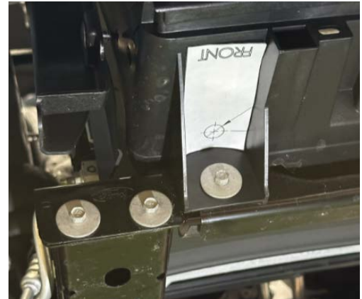
Passenger Side template location
