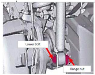
6. Remove shock absorbers and springs from vehicle. Discard hardware.
