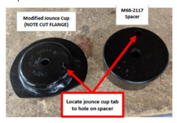
15. Apply Loctite 271 to M8 bolt before install. Install assembly on frame so cut flange faces outside of vehicle (pin on spacer will locate to rear).
