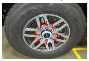
23. If vehicle is on the ground, use a shop lift or floor jack to raise the vehicle off ground and remove rear wheels, save for reuse.
