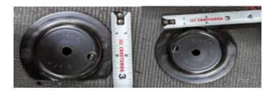
14. Assemble jounce bumper with modified jounce cup and spacer. (NOTE: 1818 will be etched into the part to identify it as the one to use)
