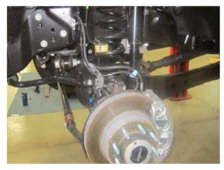
4. Remove upper shock nut, washer, and bushing on both sides of vehicle with 21 mm socket wrench. Discard hardware.
