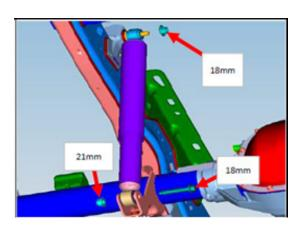
25. Install new shocks (986-24-097) and fasten nut at upper location with 18mm socket wrench. Torque to 70 Nm.
