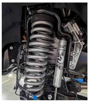
8. Install new shocks (986-24-098) and fasten lower bolts and flange nuts with 18mm socket wrench. Torque to 150 Nm.
