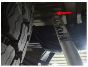
26. Fasten shocks at lower location with nut and bolt and 18mm and 21mm socket wrenches. Torque to 150 Nm.
