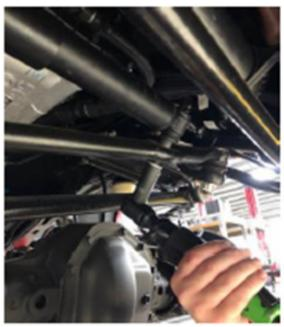
18. Subassemble fastener set provided in the steering stabilizer kit 986-24-099. Long end of the bolt goes through stabilizer. Tighten rear nut using 19mm socket.
