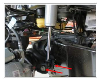
9. Install upper shock nuts with 21mm socket wrench and torque to 61 Nm.
