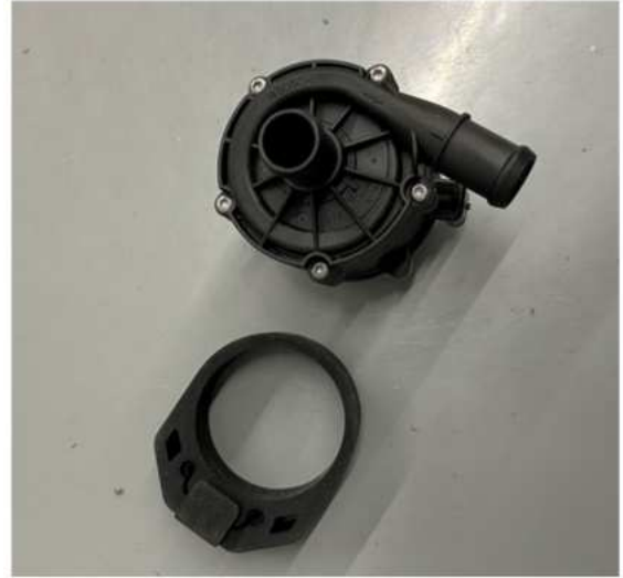
Intercooler pump and grommet facing up orientation
