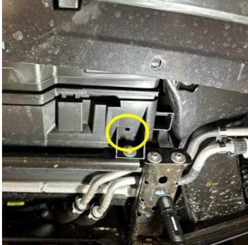
Driver Side cut hole
