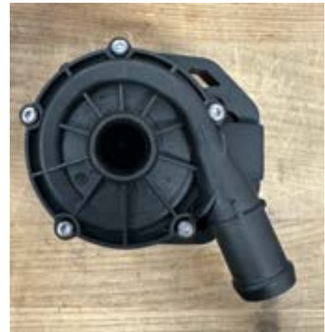
Intercooler pump sub-assembly_Top View
