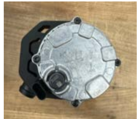
Intercooler pump sub-assembly_Bottom View
