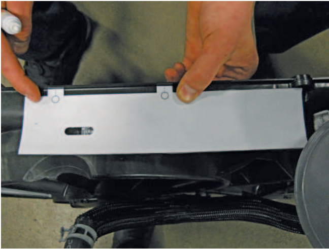
Proper template position on fan shroud
