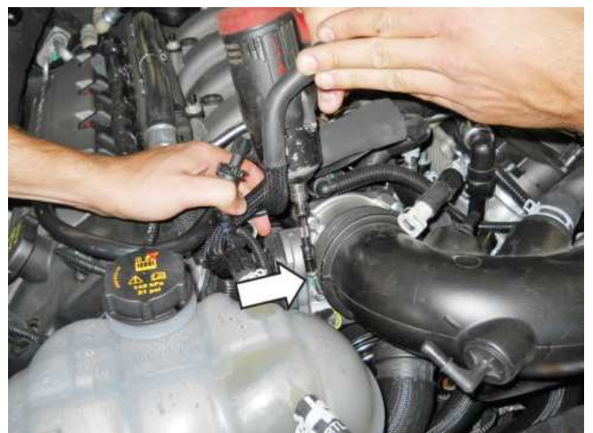
Clamp at throttle body
