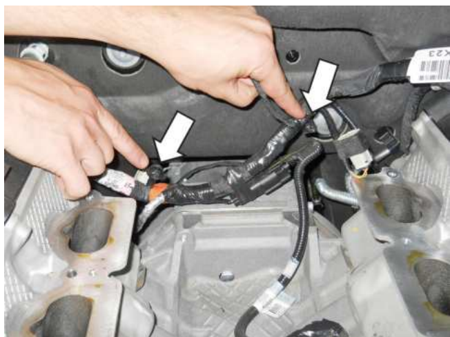
Pin retainers on harness
