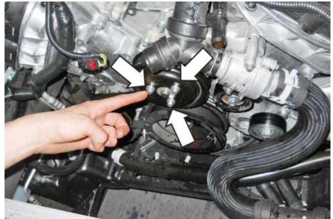
43. Cut and remove the A/C compressor belt. Discard the belt.
