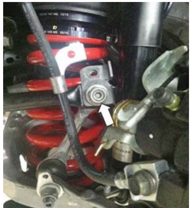
14. Use an 18 mm box-end wrench and a 6 mm hex bit to refasten the sway bar end link bolt nut. Torque to 115 Nm.
