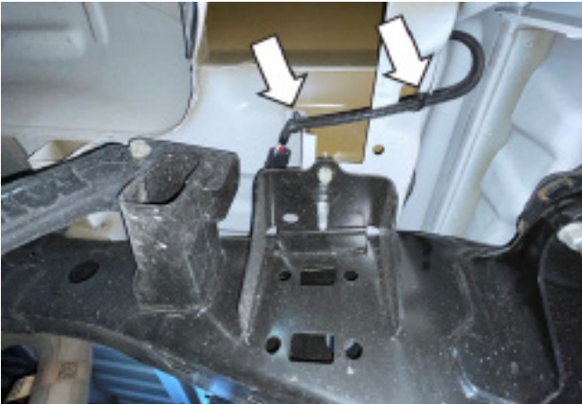
10. Pull any slack in the wire harness back through the vent and secure the wire harness.
